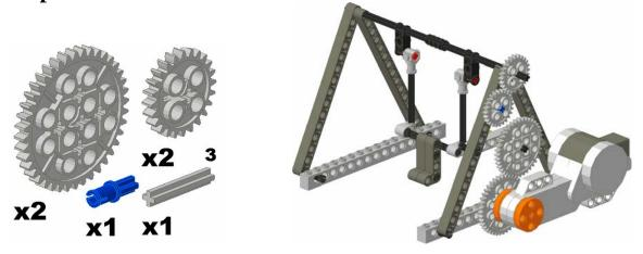
Place one of the 24 tooth gears on the exposed 10 stud axle at the top of the assembly. Connect the other 24 tooth gear using the axle pin to the 4<sup>th</sup> hole from the top of the beam. Connect one of the 40 tooth gears to the 5 stud axle in the middle of the assembly. Connect the other 40 gear using the 3 stud axle to the motor.
