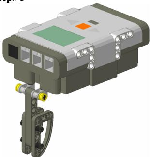
Take one of the ½ bushes off the axle and pull the axle out. Slide it back in, inserting it through the setup from step two. Replace the bush on the axle.
