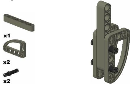
Fasten two curved beams to a 7-beam using extended pins. This is the sliding piece.
