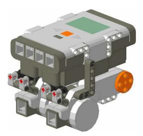
Attach each motor assembly to the bottom of the NXT by the black axle joiner, using a friction pin. Then secure each motor using the bent beam.
