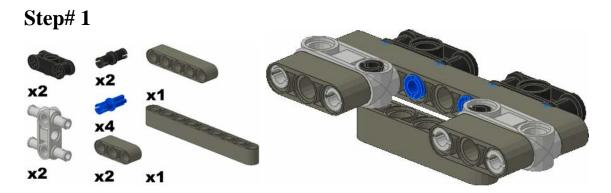
Connect the two black axle joiners to the 9-beam using the axle pins. Connect the two gray axle joiners to the 9-beam as well. Connect the 5-beam to the grey axle joiners using the connecting pins. Connect the 3-beams to the grey axle joiners.
