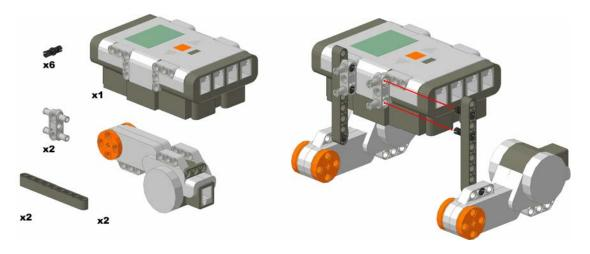
In the diagram above, the right motor and beam is extended out, to provide an intermediary step.
