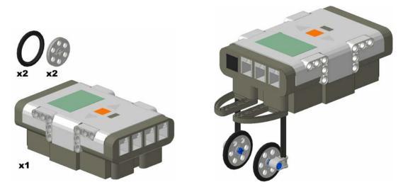
Attach each axle assembly to the NXT and add wheels to the axle pins.
